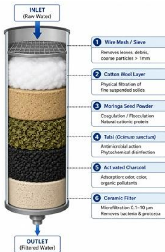
Figure 1: Schematic Cross-Section of the Multi-Layer Filtration Column (Top to Bottom)
